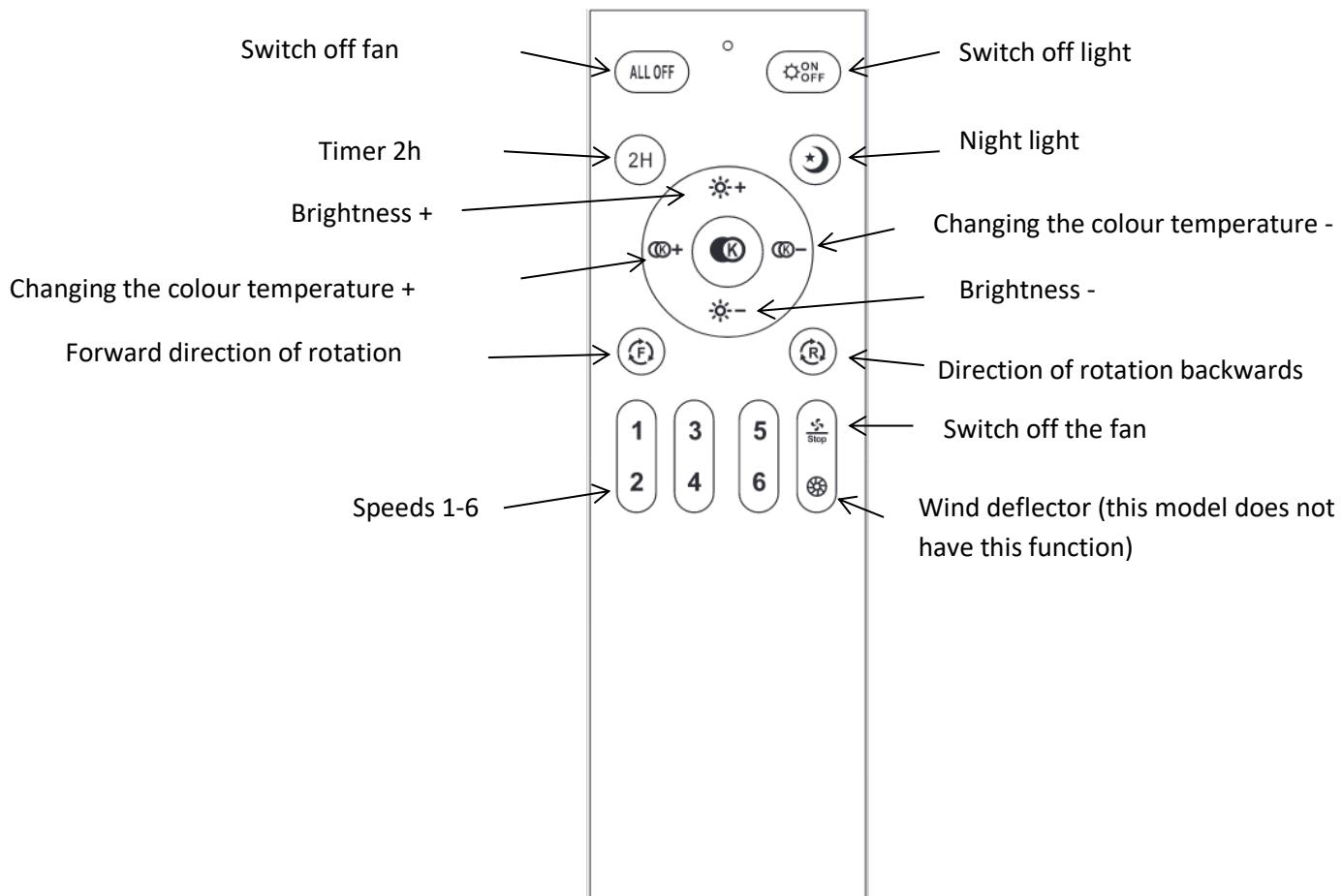
The remote control requires no special pairing and can be used as soon as the fan is installed.
