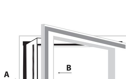
**2 EN** Attach the other half of the strap either to the inner or outer part of window casement. The window must be able to be closed.
