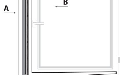
**3 EN** Keep the window open and with the zipper closed attach the wider side A to the strap on the frame. Start from the middle and continue towards the sides.
