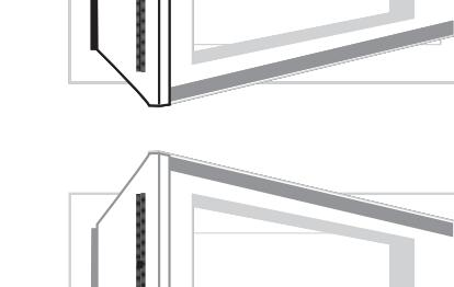
**4 EN** Close the window and make sure the seal is not pinched between the frame and the casement.
